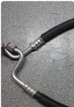
AIR CONDITION HOSE
